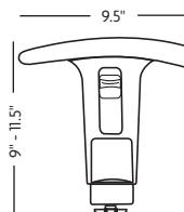
Height adjustable "T" arm with soft KIDNEY shaped urethane arm pad.
