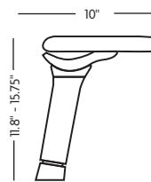
360° arm pad rotation and 360° pad base rotation with inside/outside function. Arm pad depth slide front/back. Height adjustable
