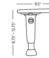
Height adjustable "T" arm with soft urethane arm pad with 360° swivel.
